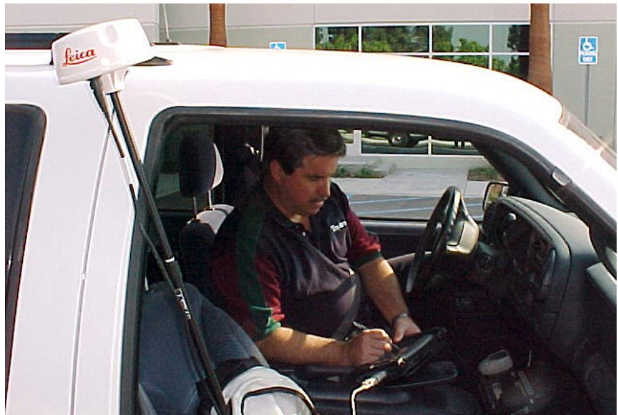
Deputy Sheriff A.D. Hall uses a Leica GS5+ to assign GPS coordinates to addresses in the City of Industry, California.
