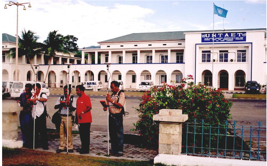
Locals use Leica's GS50 GPS/GIS receiver to record GPS coordinates of schools in East Timor.
